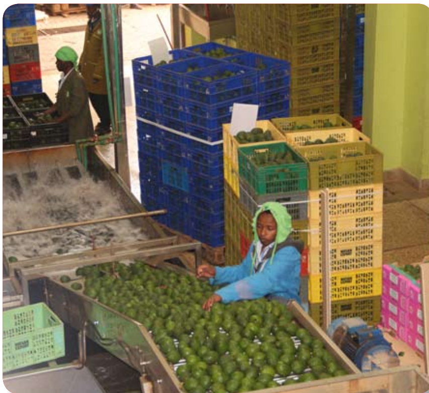
Avocados being cleaned by a machine that grades them according to their sizes at the company's packhouse
