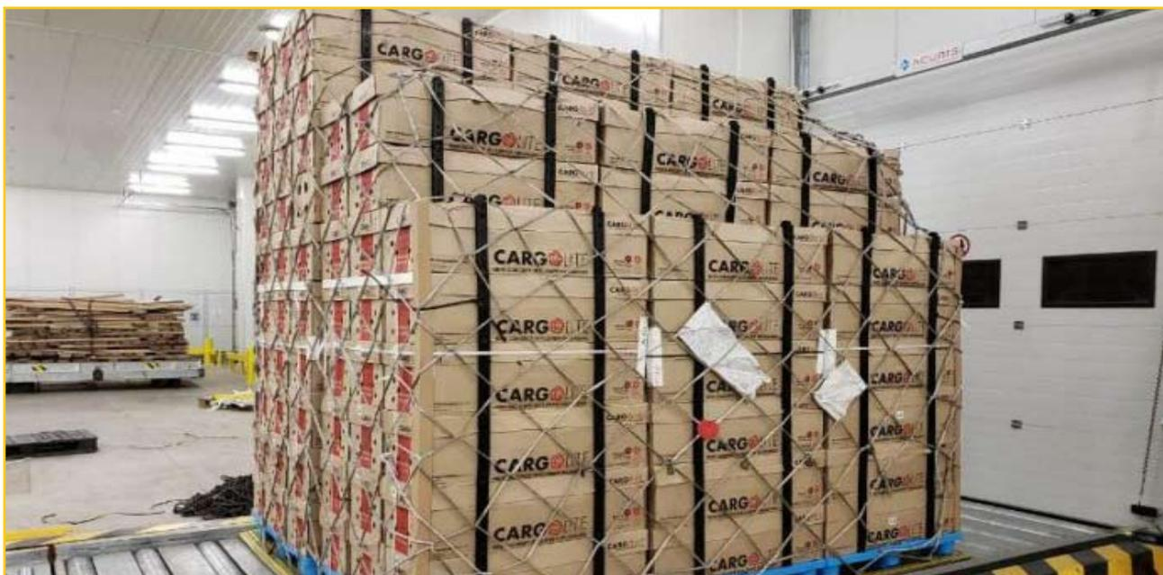
Completed air pallets with cartons neatly arranged in layers. The black frames form a supporting system that diverts the load from the carton walls to the frames.
